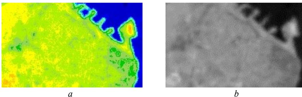
Fig. 2 Thermal field of enhanced detaility (*a*) in comparison with the original TIRS image (*b*)
